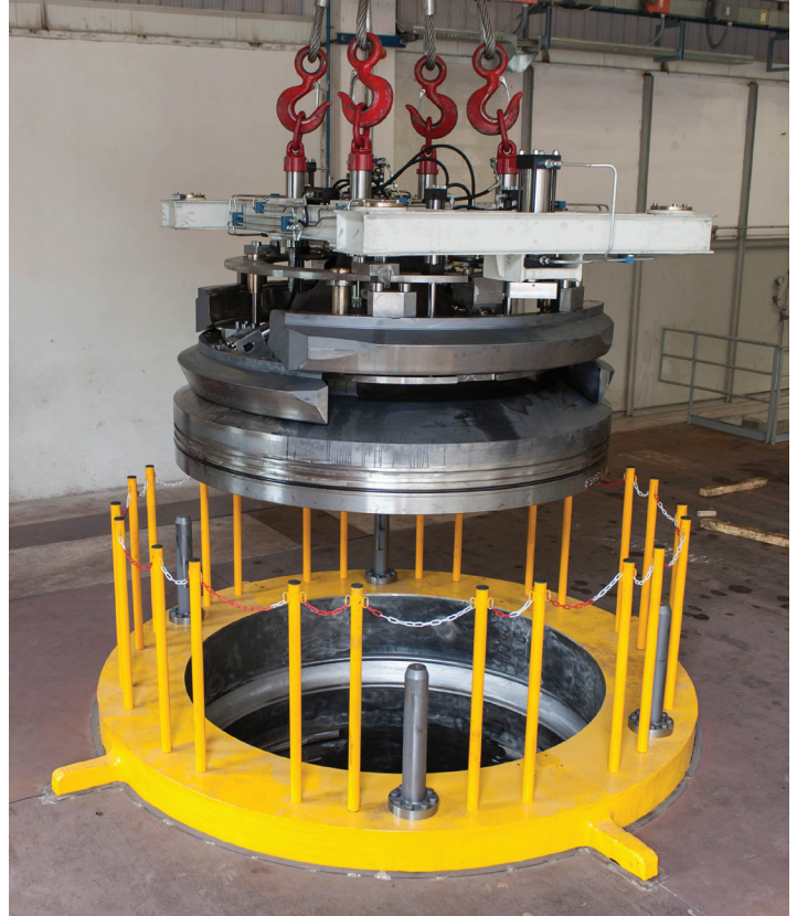
The RING-O subsea valve design is similar to equivalent topside valves, but has additional features to withstand the external pressure caused by the column of seawater at operating depths.
